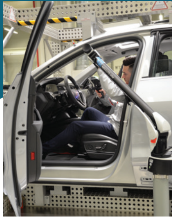
Switching from probing to scanning in the blink of an eye, the large Absolute Arm allows easy and accurate measurement inside or outside the car.
