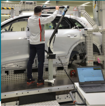
Switching from probing to scanning in the blink of an eye, the large Absolute Arm allows easy and accurate measurement inside or outside the car.
